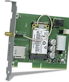
Fig. 1.6. Digicom 3G Modem USB Internal
